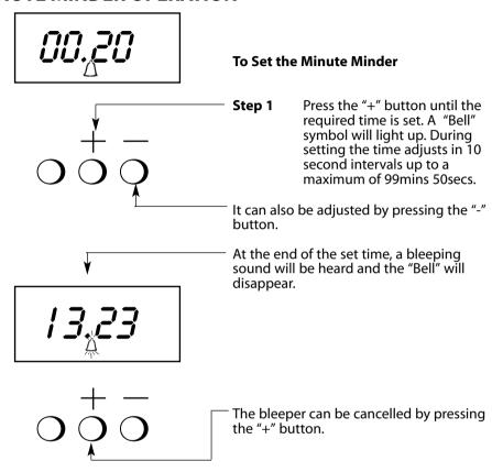
The minute minder can be cancelled before the bleeper sounds by pressing the "+" and "-" buttons together until 0.00 appears in the display window.
